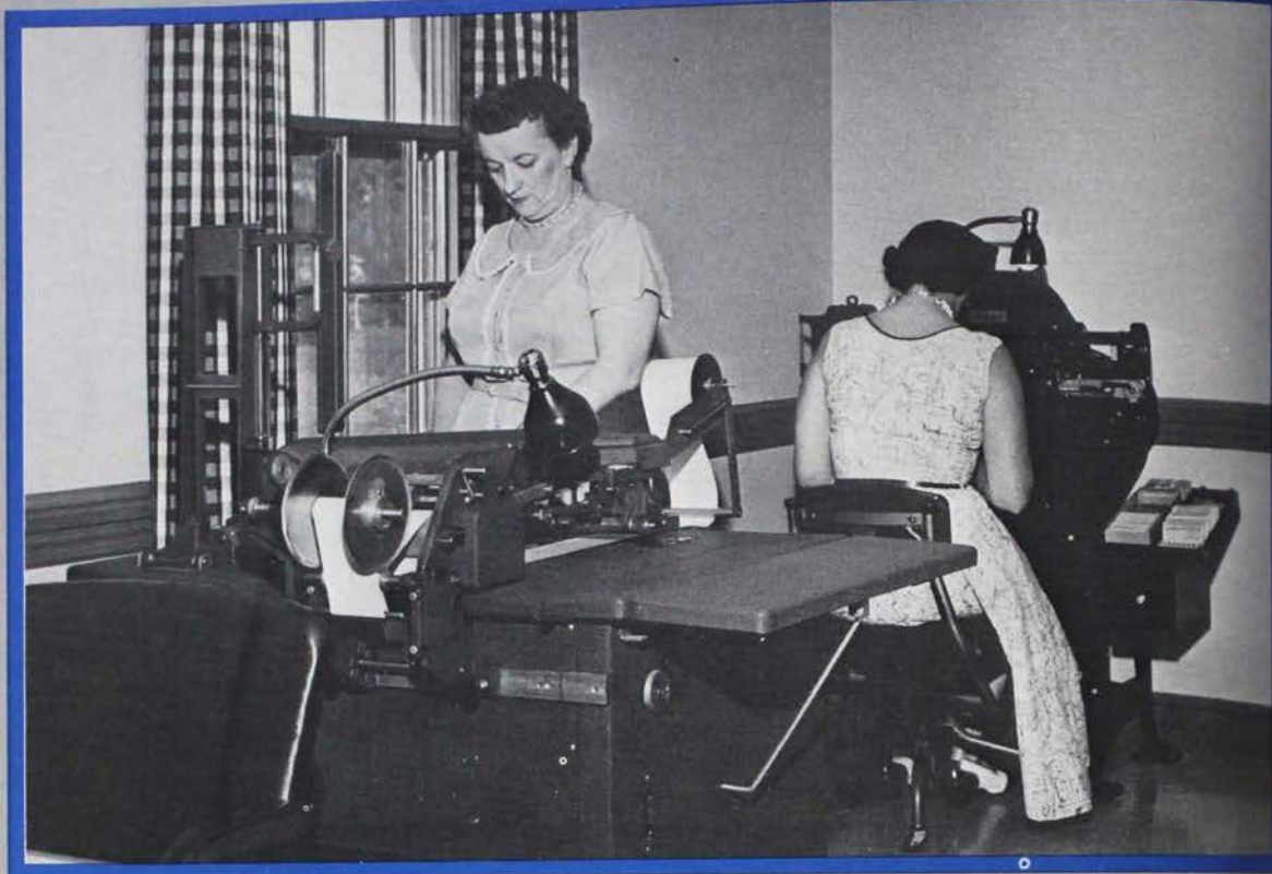
For many years prior to the use of the computer, The Central Office used addressograph machines for mass mailings.
